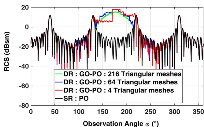
Fig. 7. Monostatic RCS of a PEC dihedral corner reflector at 10 GHz (first approach).
