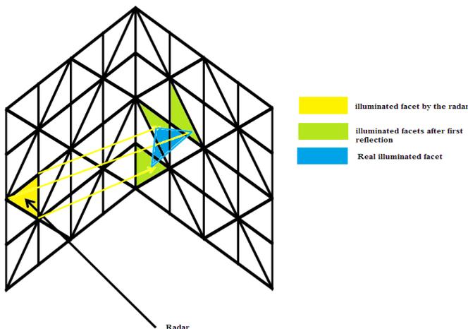
Fig. 3. Ray-triangle intersection principle.
