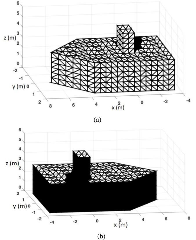
Fig. 2. Shadowing effect for an observation direction given by  $\theta = \varphi = 45^\circ$ : (a) visible facets and (b) hidden facets.
