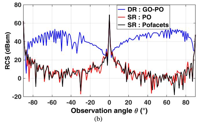
Fig. 10. Monostatic RCS of the PEC generic boat at 10 GHz (with multiple scattering): (a)  $\varphi=0^\circ$  and (b)  $\varphi=90^\circ$ .
