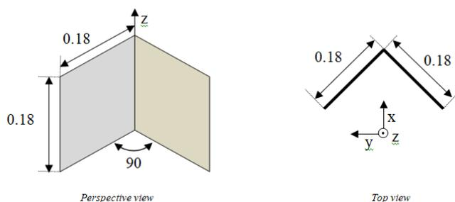
Fig. 5. The PEC dihedral corner reflector geometry and dimensions.
