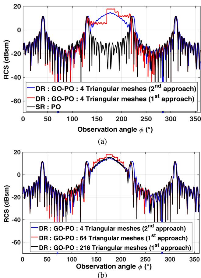
Fig. 8. Monostatic RCS of a PEC dihedral corner reflector at 10 GHz (first and second approaches).
