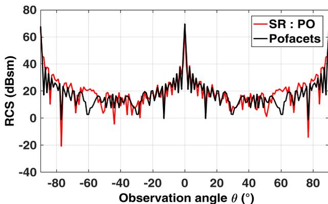
Fig. 9. Monostatic RCS of the PEC generic boat at 10 GHz (without multiple scattering):  $\varphi=90^\circ$ .
