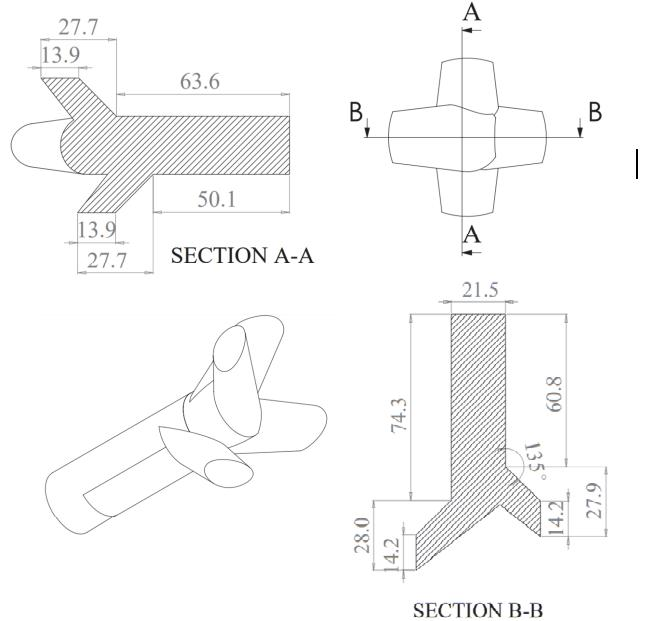
Fig. 4. Final dimensions of CPMCA
