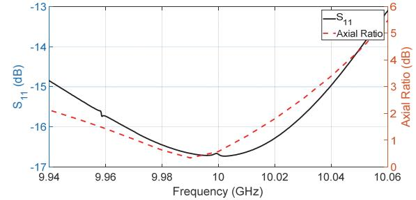
Fig. 6. The return loss and the axial ratio of the CPMCA in frequency
