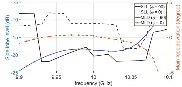
Fig. 5. The sidelobe level (SLL) and main lobe deviation of the CPMCA in the horizontal ( $\phi = 0^\circ$ ) and vertical ( $\phi = 90^\circ$ ) plane
