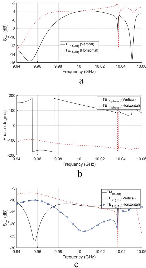
Fig. 5. The absolute and phase of the modes in the aperture: (a) the absolute and (b) phase of the  $S_{21}$  parameter of two main modes, and (c) the absolute of the three unwanted modes.
