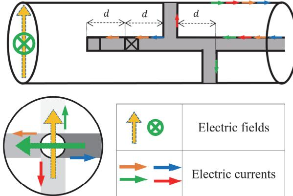
Fig. 2. Electric currents, magnetic and electric fields in the circular left-handed CPMCA
