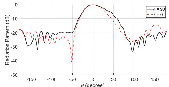
Fig. 9. The left-handed radiation patterns of the CPMCA gain at  $10$  GHz frequency, in the horizontal and vertical planes
