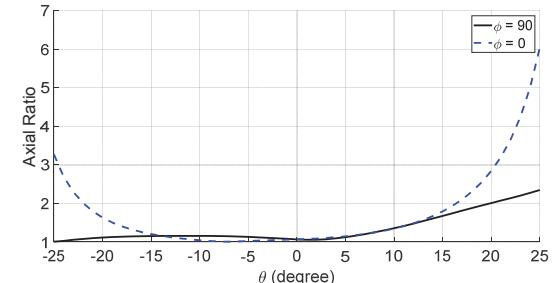
Fig. 8. The axial ratio in degree at  $10$  GHz frequency
