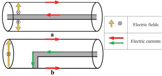
Fig. 1. Electric currents, magnetic and electric fields (a) in the coaxial waveguide and (b) in the proposed structure
