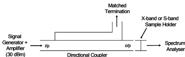
Fig. 5. Experimental setup for measurement of shielding effectiveness using a directional coupler
