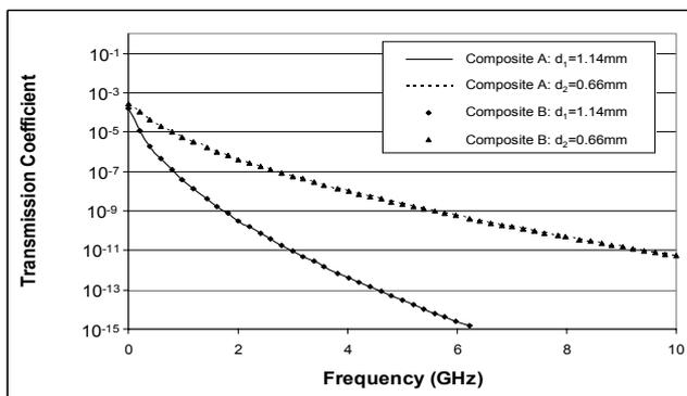
Fig. 3. Simulated transmission coefficients for CFC composites A and B for two different laminate thicknesses
