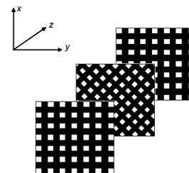
Fig. 1. Carbon Fibre Composite ply organisation (0°/45° “Composite A” or 0°/90° “Composite B”)
