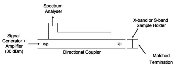
Fig. 6. Experimental setup for return loss measurement of CFC samples
