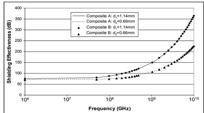
Fig. 4. Composite A and Composite B simulated shielding effectiveness using plane wave theory
