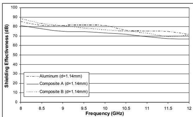
Fig. 8. Measured shielding effectiveness of the composites compared to Aluminium at X-band.
