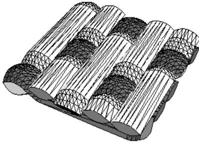
Fig. 2. CFC Laminate with 7  $\mu\text{m}$  fibre tow bundles (satin weave)[5]
