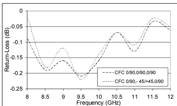
Fig. 9. Return loss for the CFC materials at X-band [9]
