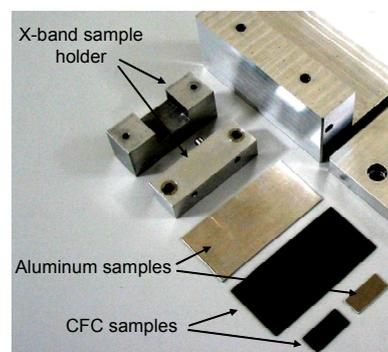
Fig. 7. Machined X-band CFC waveguide sample holder with aluminium and CFC samples
