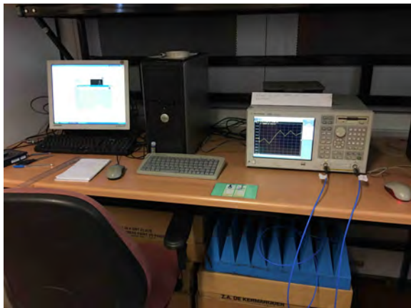
Fig. 4. Experimental set-up (PC with LabVIEW and VNA).
