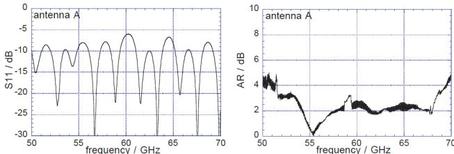
Fig. 18. Measured reflection ( $S_{11}$ ) and axial ratio (AR) of the 8x8 antenna array around 60 GHz
