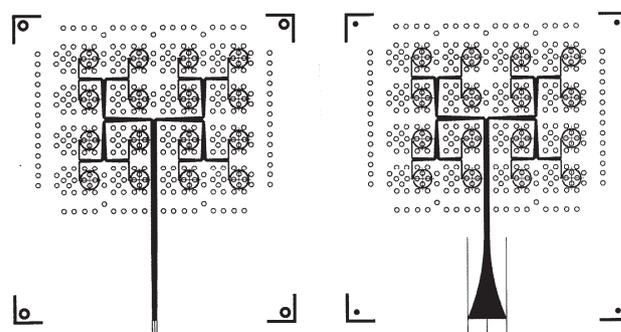
Fig. 6. Lay-out of both sides of 4x4 two-dimensional antenna array around 15 GHz with a bal-un transition
