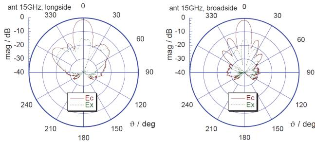
Fig. 14. Measured radiation pattern: long side and broad side cut of the 4x4 antenna array around 15 GHz
