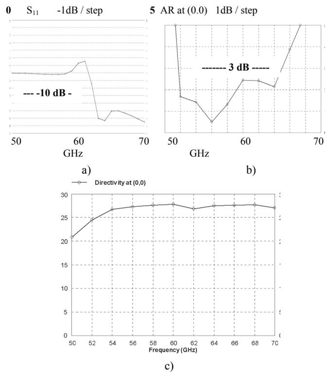
Fig. 17. Simulation results for 8x8 antenna array around 60 GHz: a)  $S_{11}$ , b) AR and c) Directivity
