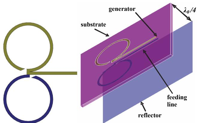
Fig. 1. The basic antenna dipole and reflector
