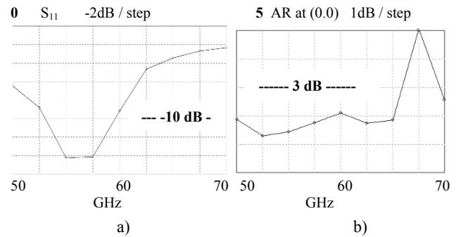
Fig. 16. Simulation results for 6x6 antenna array around 60 GHz:
