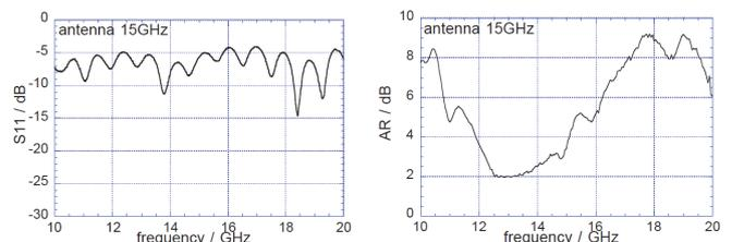
Fig. 12. Measured reflection ( $S_{11}$ ) and axial ratio (AR) of the 4x4 antenna array around 15 GHz
