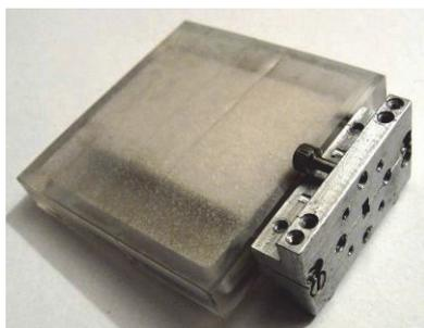
Fig. 9. Assembled 8x8 antenna array around 60 GHz: Plastic case and waveguide connector for WR-15
