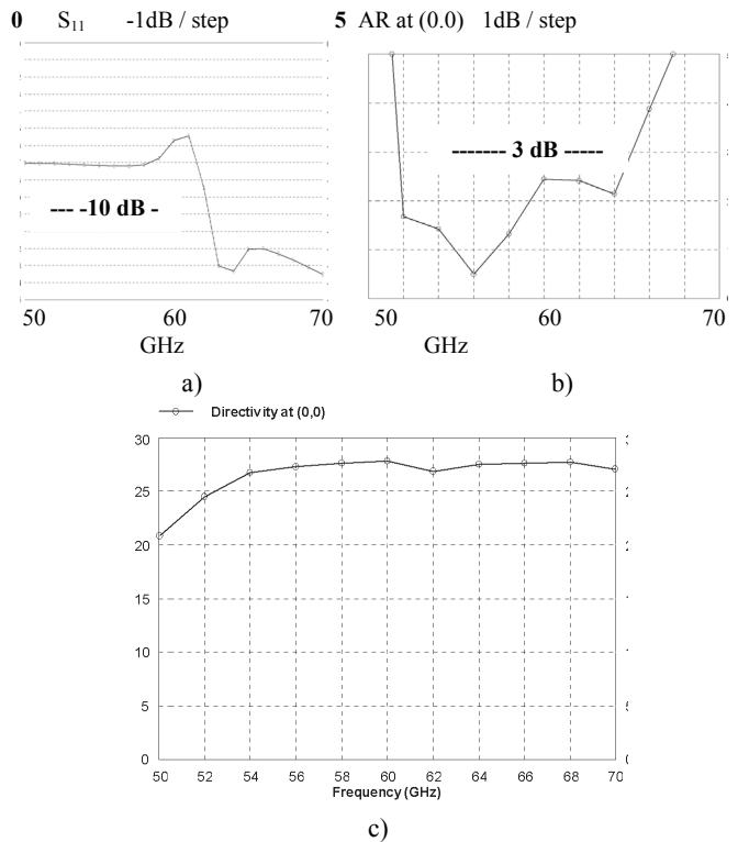
Fig. 17. Simulation results for 8x8 antenna array around 60 GHz:
