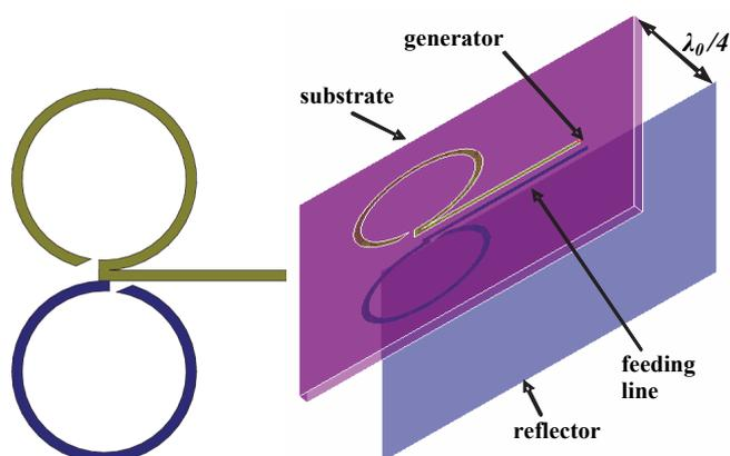
Fig. 1. The basic antenna dipole and reflector
