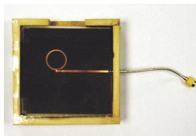
Fig. 5. Fabricated one dipole antenna around 5 GHz (upper side) with SMA connector
