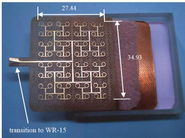
Fig. 8. Fabricated 8x8 two-dimensional antenna array around 60 GHz in parts. From up to down: antenna substrate, polyurethane foam, reflector and plastic case. Opposite open rings and feeding network are on the opposite side of the antenna substrate
