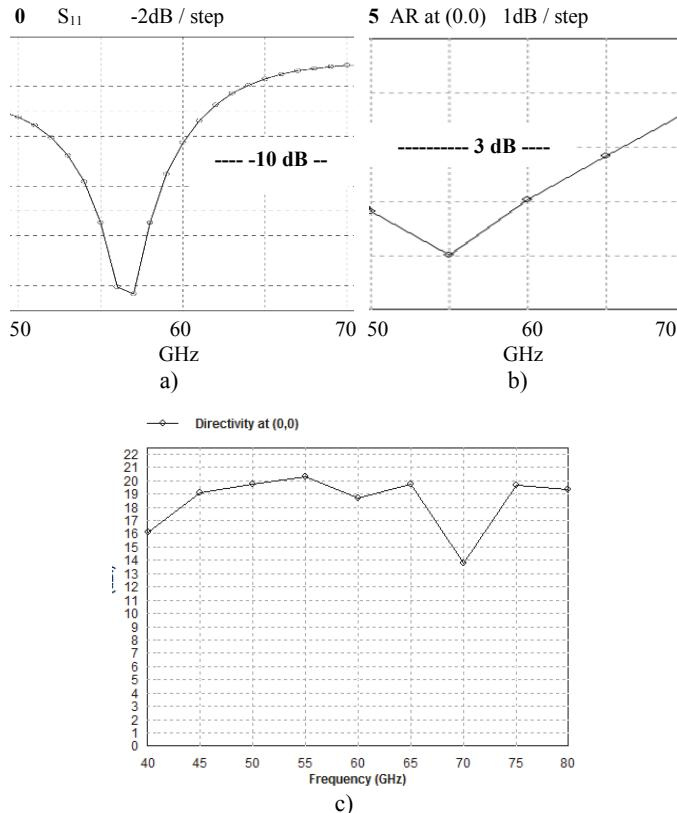
Fig. 15. Simulation results for 4x4 antenna array around 60 GHz:
