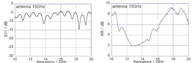
Fig. 12. Measured reflection ( $S_{11}$ ) and axial ratio (AR) of the 4x4 antenna array around 15 GHz
