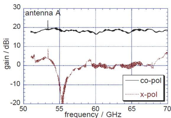
Fig. 19. Measured Gain (copolarization) and attenuation of x-polarization (opposite circulation) of the 8x8 antenna array around 60 GHz
