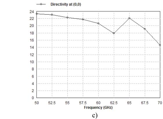
Fig. 16. Simulation results for 6x6 antenna array around 60 GHz: a)  $S_{11}$ , b) AR and c) Directivity.
