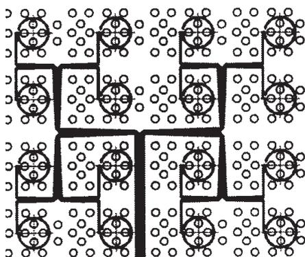
Fig. 3. An example of the feeding network: Upper side. Impedance transformers as tapered symmetrical microstrip lines
