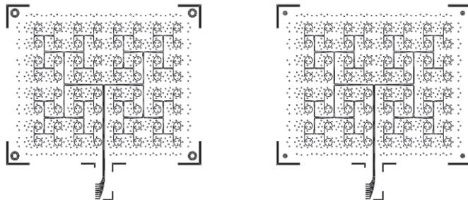
Fig. 7. Lay-out of both sides of 8x8 two-dimensional antenna array around 60 GHz with transition to waveguide
