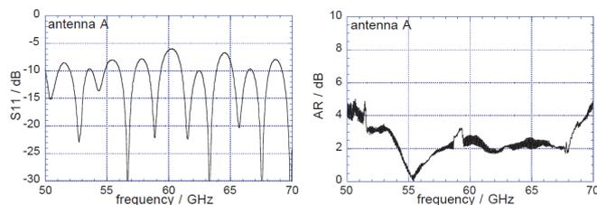
Fig. 18. Measured reflection ( $S_{11}$ ) and axial ratio (AR) of the 8x8 antenna array around 60 GHz
