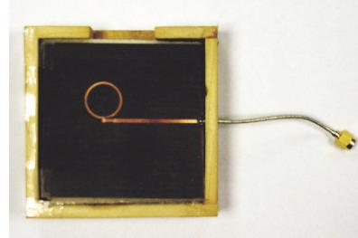
Fig. 5. Fabricated one dipole antenna around 5 GHz (upper side) with SMA connector
