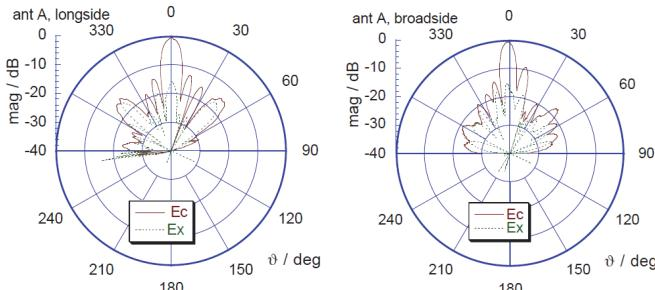
Fig. 20. Measured radiation pattern: long side and broad side cut of the 8x8 antenna array around 60 GHz
