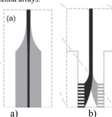
Fig. 4. Transition from symmetrical microstrip according to frequency (Black-upper side, Gray-down side): a) Bal-un transition; b) Transition to waveguide
