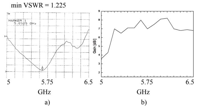
Fig. 10. Measured a) VSWR and b) gain vs frequency of the scaled realized model of the double open ring tapes around 5 GHz
