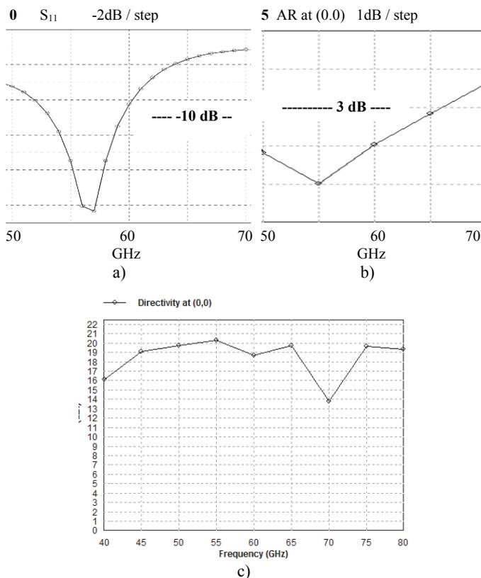
Fig. 15. Simulation results for 4x4 antenna array around 60 GHz: a)  $S_{11}$ , b) AR and c) Directivity
