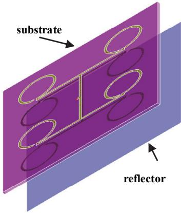
Fig. 2. Basic concept of a simple 2x2 two-dimensional antenna array with a reflector
