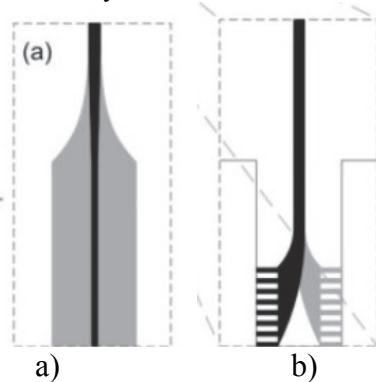
Fig. 4. Transition from symmetrical microstrip according to frequency (Black-upper side, Gray-down side):
