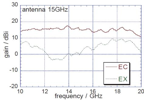
Fig. 13. Measured Gain (copolarization) and attenuation of x-polarization (opposite circulation) of the 4x4 antenna array around 15 GHz
