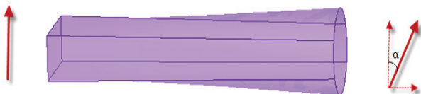
Fig. 2. Circular to rectangular waveguide transition and polarization rotation
