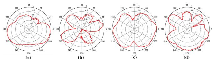
Fig. 11. Measured radiation pattern of Antenna 2 at frequency 9 GHz: (a) E-plane co-pol, (b) E-plane cross-pol, (c) H-plane co-pol, and (d) H-plane cross-pol
