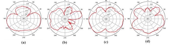
Fig. 12. Measured radiation pattern of Antenna 3 at frequency 9 GHz: (a) E-plane co-pol, (b) E-plane cross-pol, (c) H-plane co-pol, and (d) H-plane cross-pol
