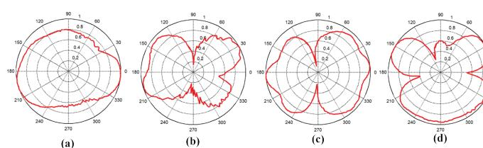
Fig. 10. Measured radiation pattern of Antenna 1 at frequency 9 GHz: (a) E-plane co-pol, (b) E-plane cross-pol, (c) H-plane co-pol, and (d) H-plane cross-pol
