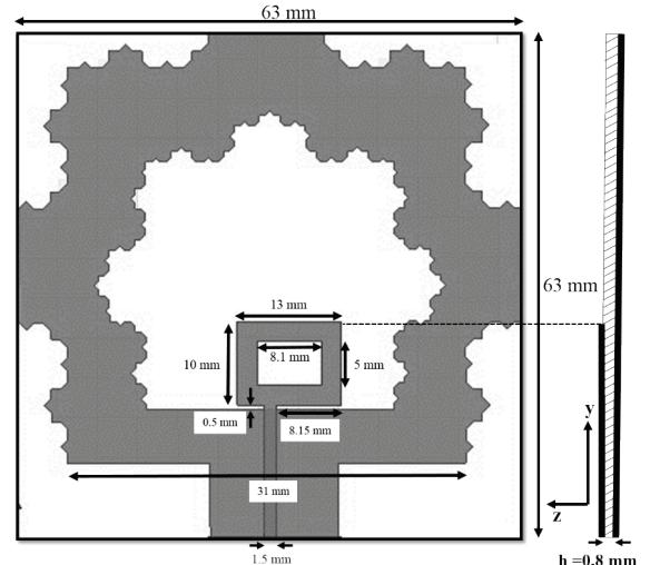
Fig. 3. Configuration of the proposed slot antenna (Antenna3)
