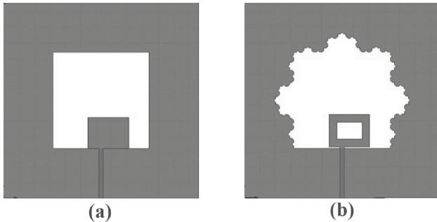
Fig. 2. Antenna configurations: (a) Initial square slot antenna (Antenna 1) [1], (b) Koch fractal slot antenna (Antenna 2) [1]
