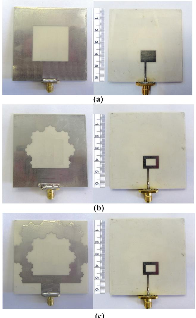
Fig. 7. Fabricated antennas on RO4003: (a) Antenna 1, (b) Antenna 2, and (c) Antenna 3
