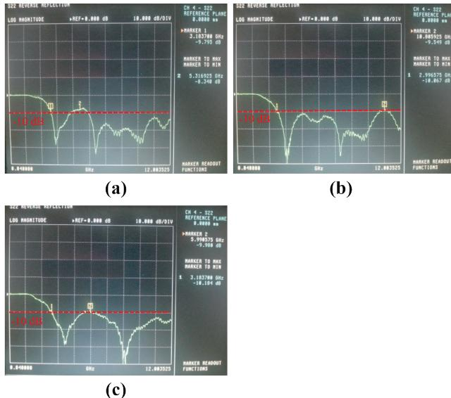
Fig. 8. Measured return loss of the three antennas: (a) Antenna 1, (b) Antenna 2, and (c) Antenna 3
