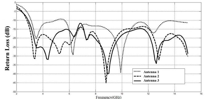
Fig. 4. The impedance bandwidth comparison of the three antennas
