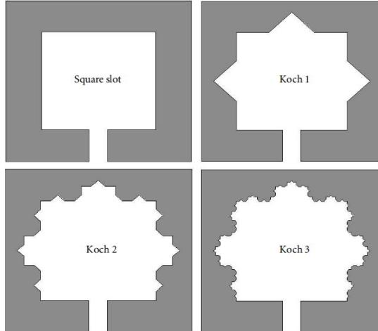
Fig. 1. Geometry of the square slot and three modified Koch slots with different iterations [2]
