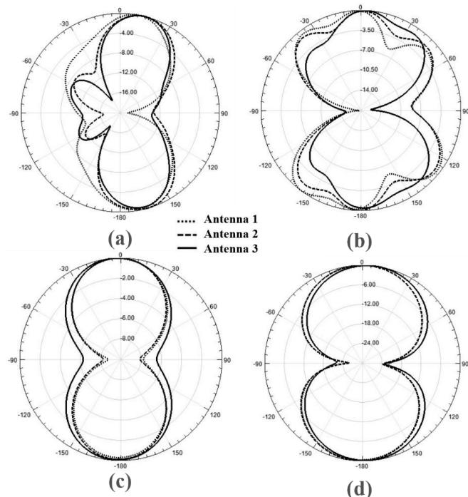
Fig. 6. Simulated radiation patterns of the three antennas: (a) 9 GHz H-plane, (b) 9 GHz E-plane, (c) 3 GHz H-plane, (d) 3 GHz E-plane
