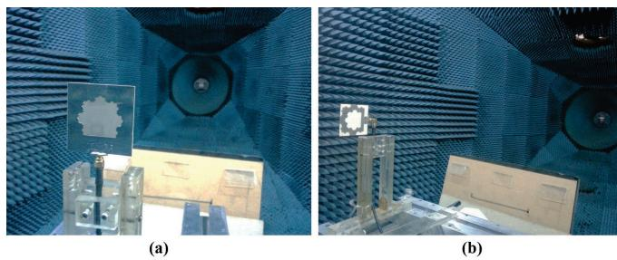
Fig. 9. Radiation pattern measurement of the three antennas:
