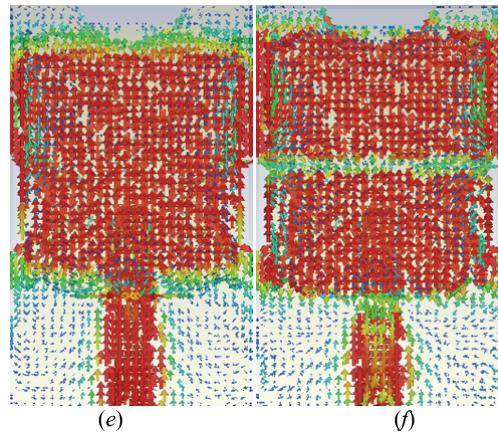
Fig. 3. (a) Back view of the proposed antenna, (b)  $S_{11}$  parameter, (c) gain at 2.4 GHz, (d) gain at 4.7 GHz, (e) current distribution at 2.4 GHz, and (f) current distribution at 4.7 GHz
