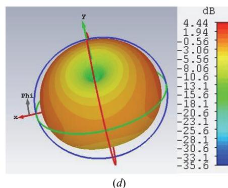
Fig. 2. (a) Slot cutting dual layer antenna, (b)  $S_{11}$  parameter, (c) gain at 2.4 GHz, and (d) gain at 4.7 GHz
