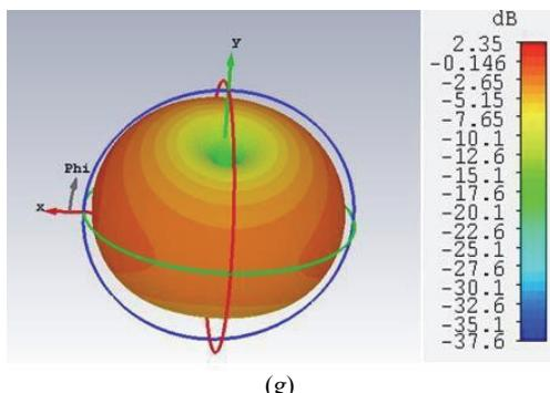
Fig. 1. (a) Proposed single layer antenna, (b) proposed dual layer antenna, (c) stacked proposed design, (d)  $S_{11}$  result single layer antenna, (e)  $S_{11}$  result dual layer antenna, (f) gain of the single layer antenna, and (g) gain of the dual layer antenna
