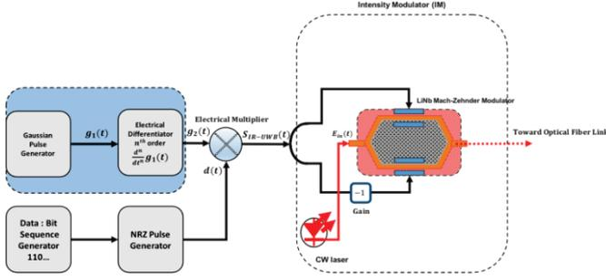
Fig. 4. The SP IR-UWB transmitter (inset in the block (e) at Fig. 1)
