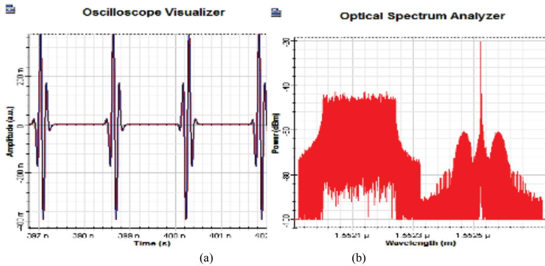
Fig. 9. The time waveform of IR-UWB based on BPM (a) and the optical spectrum of the DP CO-OFDM with SP IR-UWB (b)
