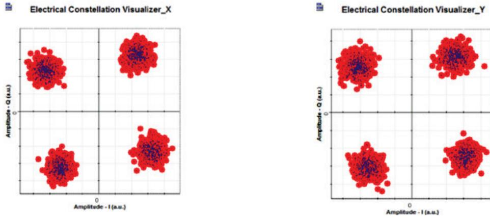
Fig. 12. The received constellation diagram at the DP CO-OFDM demodulators
