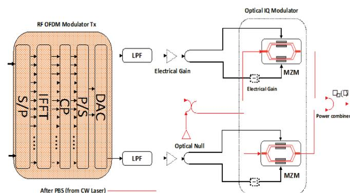
Fig. 2. The CO-OFDM transmitter
