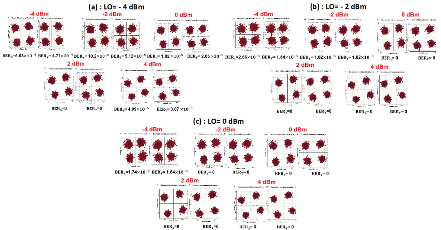
Fig. 7. Constellation diagram of post compensation at different input and LO powers
