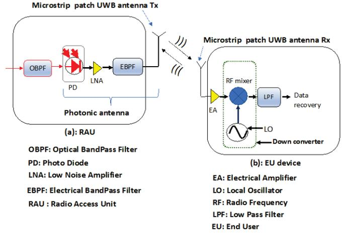
Fig. 5. The SP IR-UWB receiver with the end user device (inset in the block (f) and (g) at Fig. 1)
