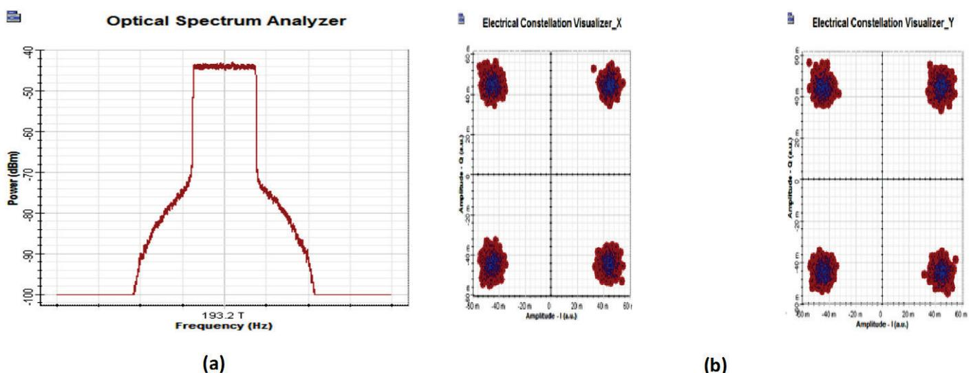
Fig. 6. The optical spectrum (a) with the received back-to-back constellation diagrams (b) of the optical OFDM signal
