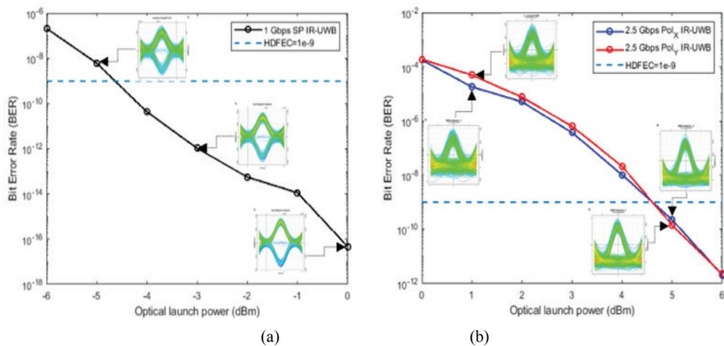
Fig. 11. BER for SP IR-UWB BPM (a) and DP IR-UWB OOK (b) (Insets: corresponding eye diagrams)
