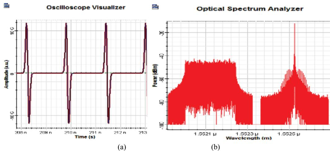
Fig. 10. The time waveform of IR-UWB based on OOK (a) and the optical spectrum of the DP CO-OFDM with DP IR-UWB (b)
