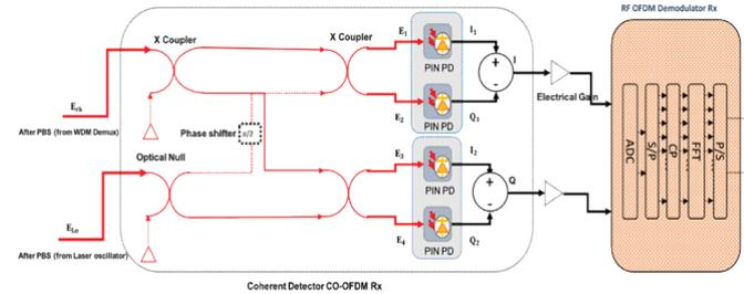
Fig. 3. The CO-OFDM receiver
