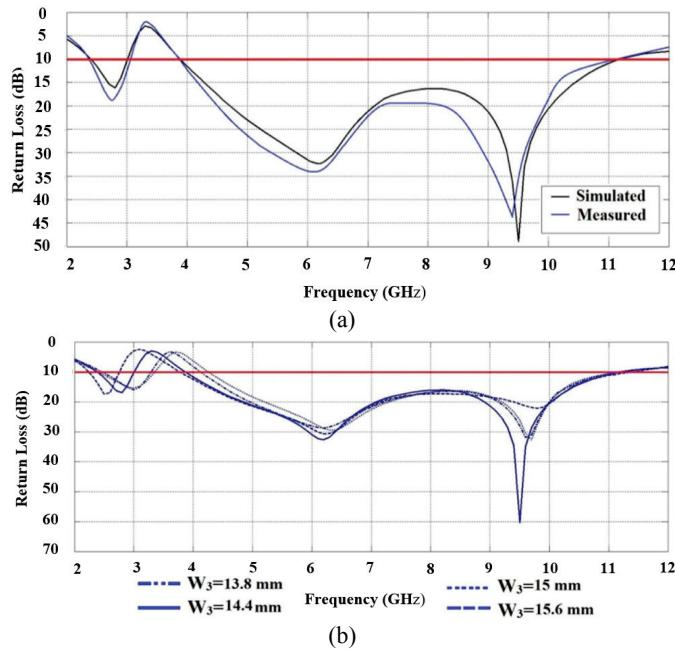
Fig. 6. (a) Simulated return loss of the proposed antenna for WIMAX band rejection with different values of  $W_3$ , (b) Measured and simulated return loss of the antenna for WIMAX band rejection
