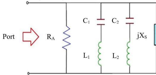
Fig. 2. Equivalent circuit of the proposed antenna around the notch band
