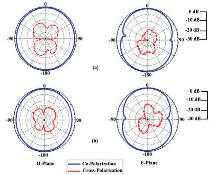
Fig. 8. Measured radiation patterns of the fabricated antenna: (a) 4.5 GHz and (b) 7.5 GHz
