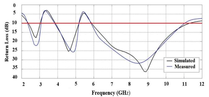
Fig. 7. Measured and simulated return loss of the dual band-notched monopole antenna
