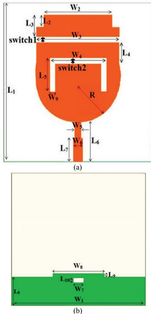
Fig. 1. Geometry of the proposed antenna (a) Top view, (b) Bottom view
