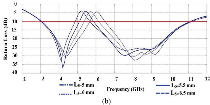
Fig. 5. (a) Measured and simulated return loss of the proposed antenna for WLAN band rejection, (b) Simulated return loss of the antenna for WLAN band rejection with different values of  $L_5$
