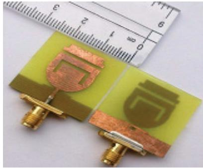
Fig. 3. Photograph of fabricated antenna
