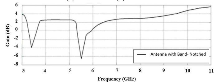
Fig. 9. Measured peak gain of the proposed antenna
