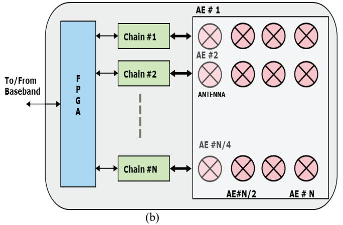
Fig. 5. Connection between LTE RRH and antenna:
