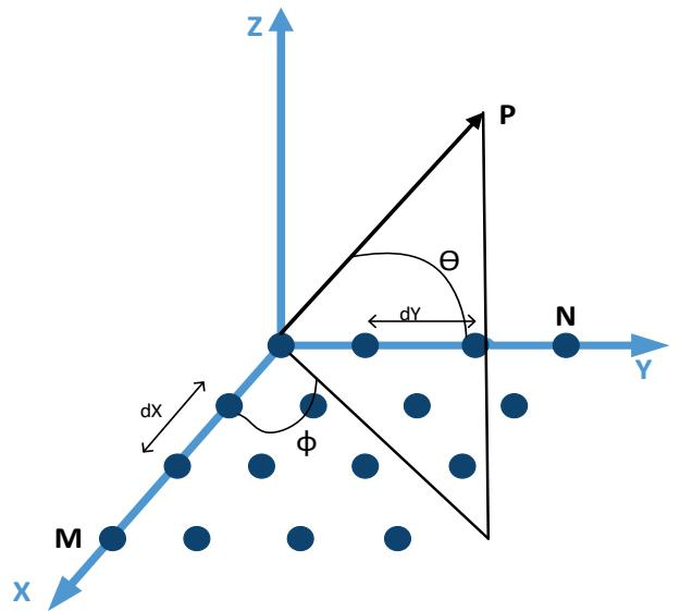
Fig. 2. Antenna array for 3-dimensional beamforming
