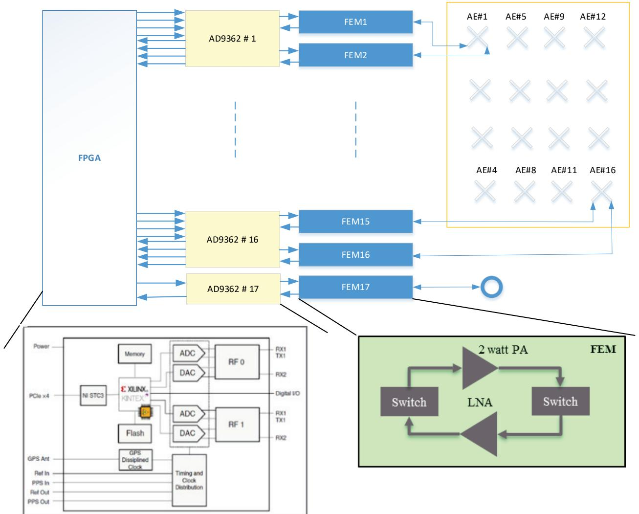
Fig. 6. Block Diagram of Massive MIMO RRH
