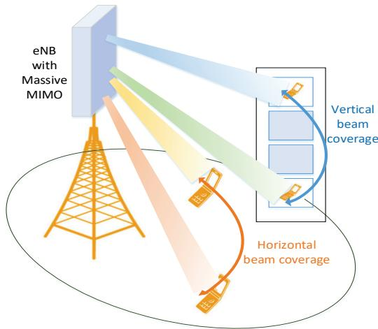
Fig. 1. Three-dimensional beamforming for massive MIMO [4]
