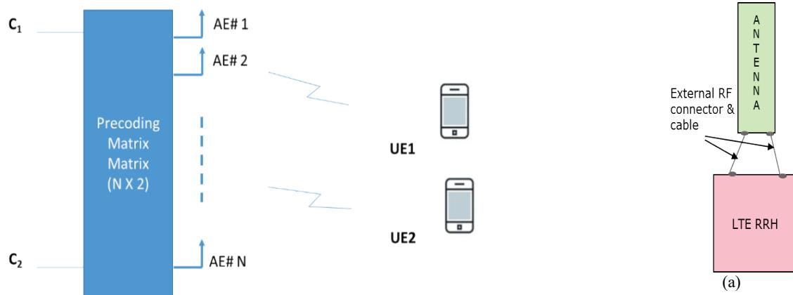
Fig. 4. Two UE downlink scenario for massive MIMO eNB
